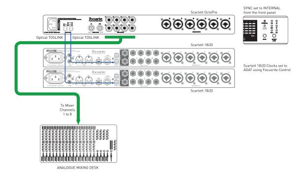
This example shows how the setup in Example 4 can be extended to add simultaneous digital recording, with or without secondary backup.
