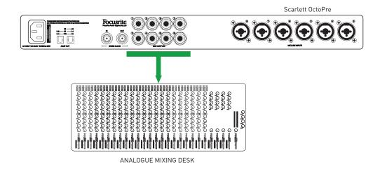
This setup uses the Scarlett OctoPre's mic pre-amplifiers to provide a high quality "front end" for an analogue mixing desk. Use a pre-made loom to connect the OctoPre's **LINE OUTPUTS** socket to eight line inputs on the mixing desk; this will need eight  $\frac{1}{4}$ " TRS jacks on one end and eight connectors appropriate to the desk's line inputs on the other. If the desk's line inputs are unbalanced, a loom with TS jacks at the OctoPre end will be suitable.
