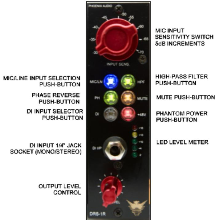
connected to the OUTPUT of the unit, NOT the mic-pre section. This makes the LED's indication much more useful for setting up levels on the Mic-Pre and the DI, and to give you a clear view of what level is being sent to external equipment.
