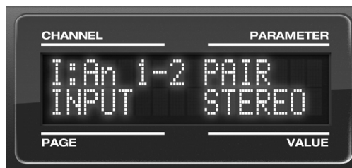
Figure 3-7: The settings for analog inputs 1 and 2 (as a pair).
