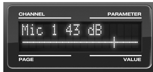
Figure 3-5: The LCD gives you feedback as you turn the TRIM knobs for the two mic/guitar inputs.
