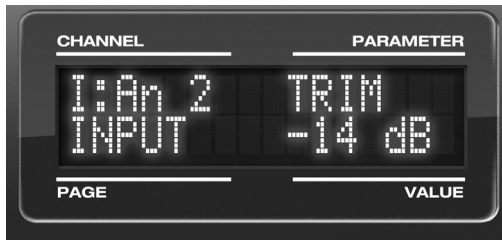
Figure 3-8: Setting the input trim for a TRS analog input pair.
