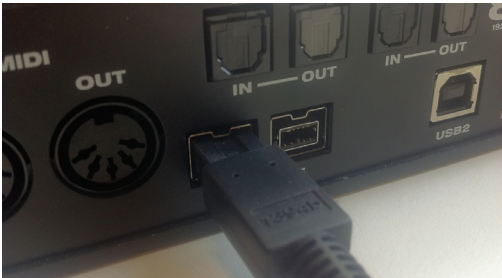
Figure 3-1: Connecting the 828mk3 to the computer via FireWire.
