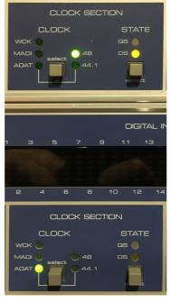
The bottom clock should always be set to correspond with the protocol associated with the DAW/Interface you are using.
