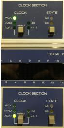
If you are working with video you may want to use the Master Clock which sends a synchronised 48K clock signal throughout the building. This is important if you want to work with a video source from somewhere else in the building but can be used for any 48k recording session as well.
