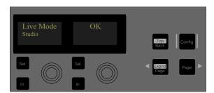
Top-row encoder displays showing mode toggle controls
