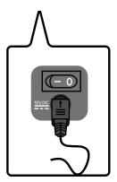
Connecting the DC power output cable to the DC In jack
