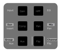
Channel Encoder Assign switches
