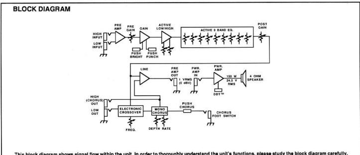
This block diagram shows signal flow within the unit. In order to thoroughly understand the unit's functions, please study the block diagram carefully.
